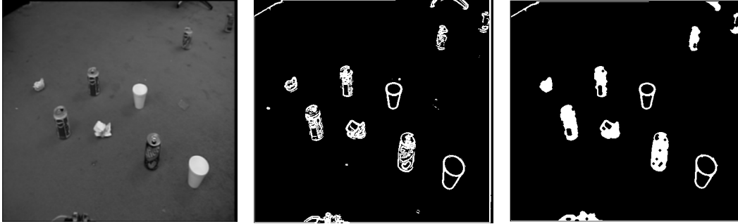
Figure 3: Trash: Raw Image, Edge Image, Filtered Image
