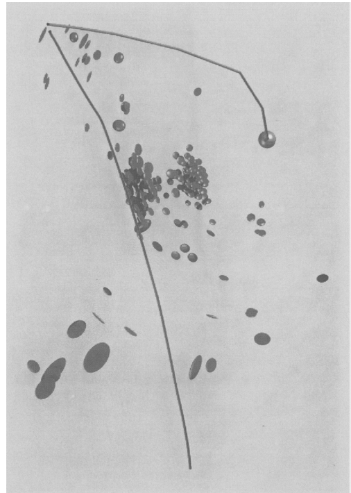
Fig. 5. Plan view of one standard deviation confidence ellipsoids for event locations in Valhall (after Dyer et al. 1999). Note clustering of event locations into two planar structures. Green sphere indicates location of geophones.
