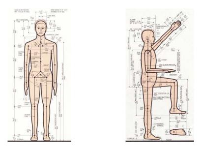
Figure 3. Front and side views of the 50<sup>th</sup> percentile proportions. Drawings from H. Dreyfuss, *The Measure of Man*, 1978.
