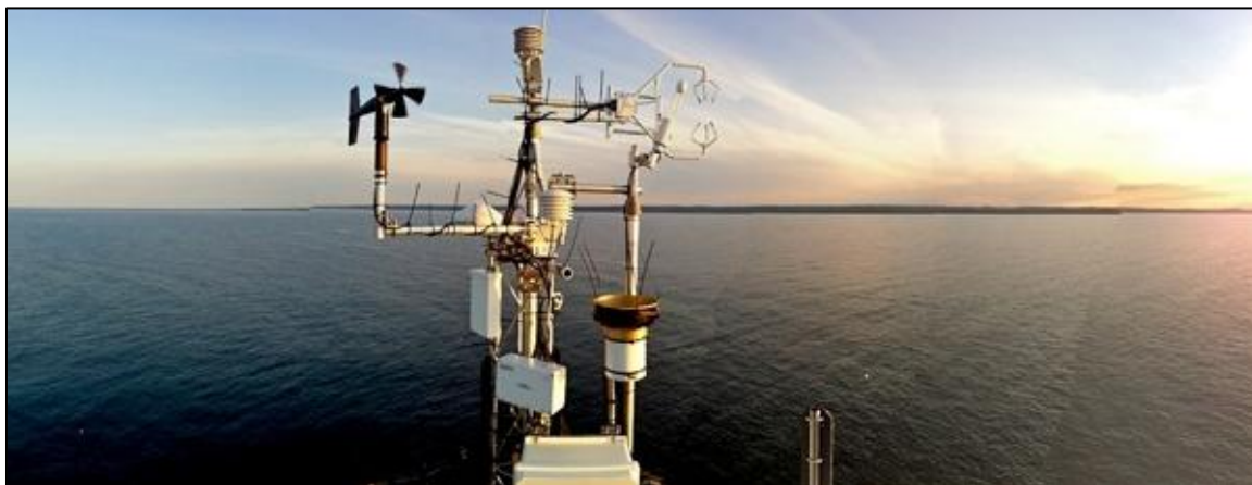
Figure 16: Granite Island flux measurement instrumentation. The LI-7500, CSAT3, and KH20 krypton hygrometer are visible in the upper right-hand corner. Additional meteorological instruments measure wind speed and direction, rainfall, barometric pressure, air temperature, humidity, and water temperature (through an infrared thermometer) (photo c/o John Lenters).
