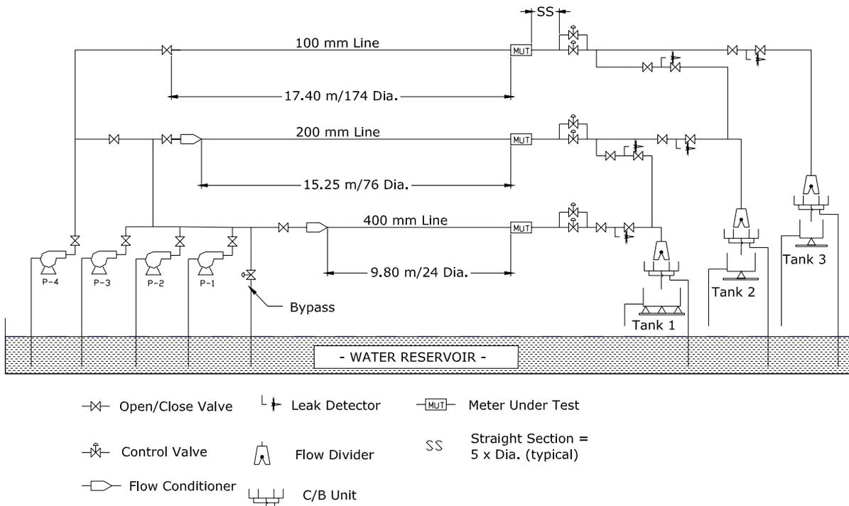
**Figure 2.** A Sketch of the Flow Paths of the Water Flow Calibration Facility.
