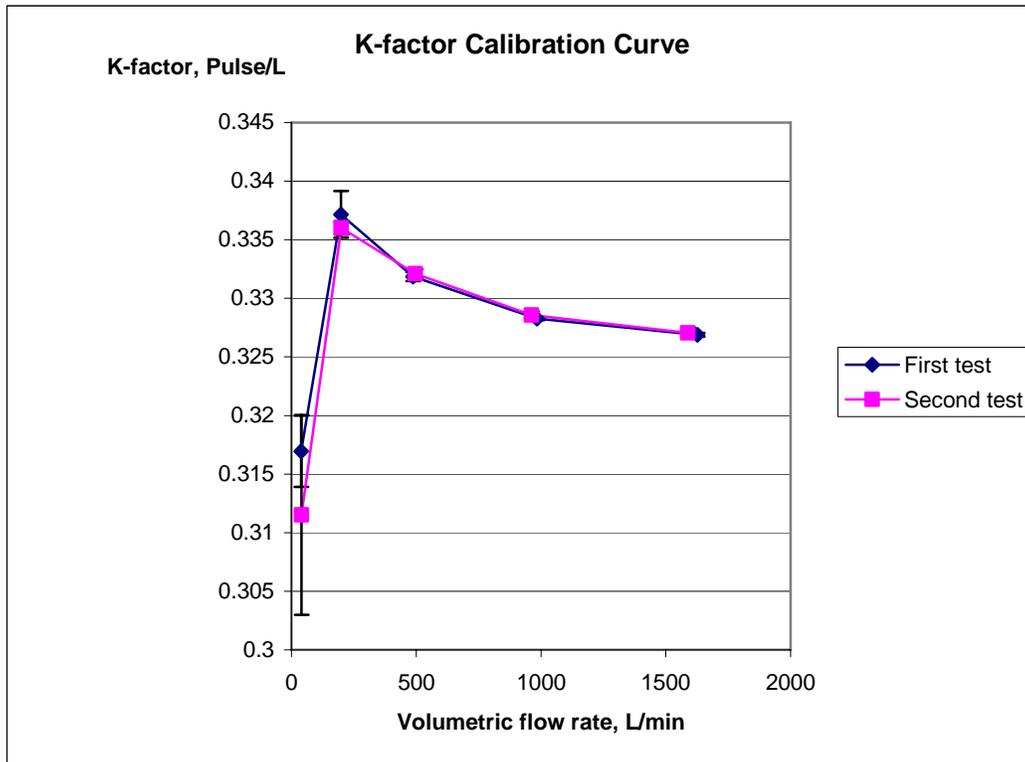
**Figure 2.** Calibration results for ABCD water flowmeter, SN 1234
