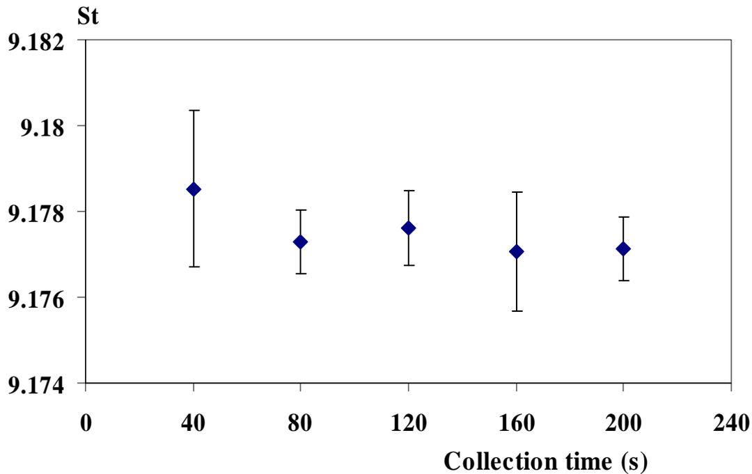
**Figure 14.** Measured Strouhal Number for Different Collection Times
