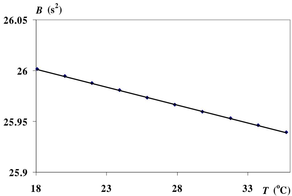
**Figure 18.** Temperature Dependence of the Densitometer Coefficient,  $B$
