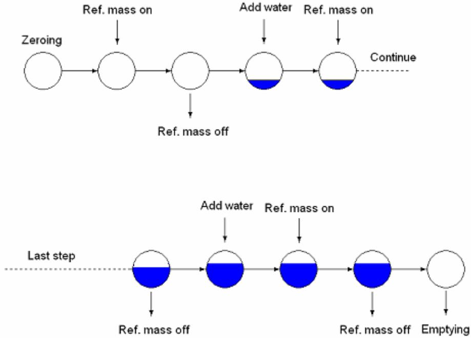
**Figure 9.** The Scale Calibration Sequence
