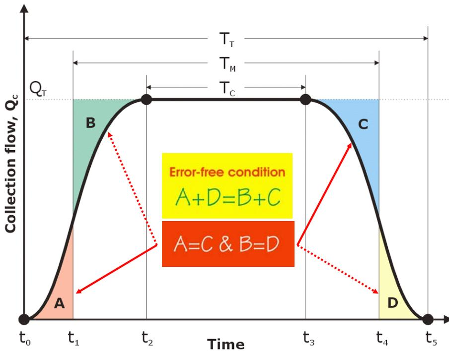
**Figure 4.** Collection Flow Diagram and Error-free Conditions.
