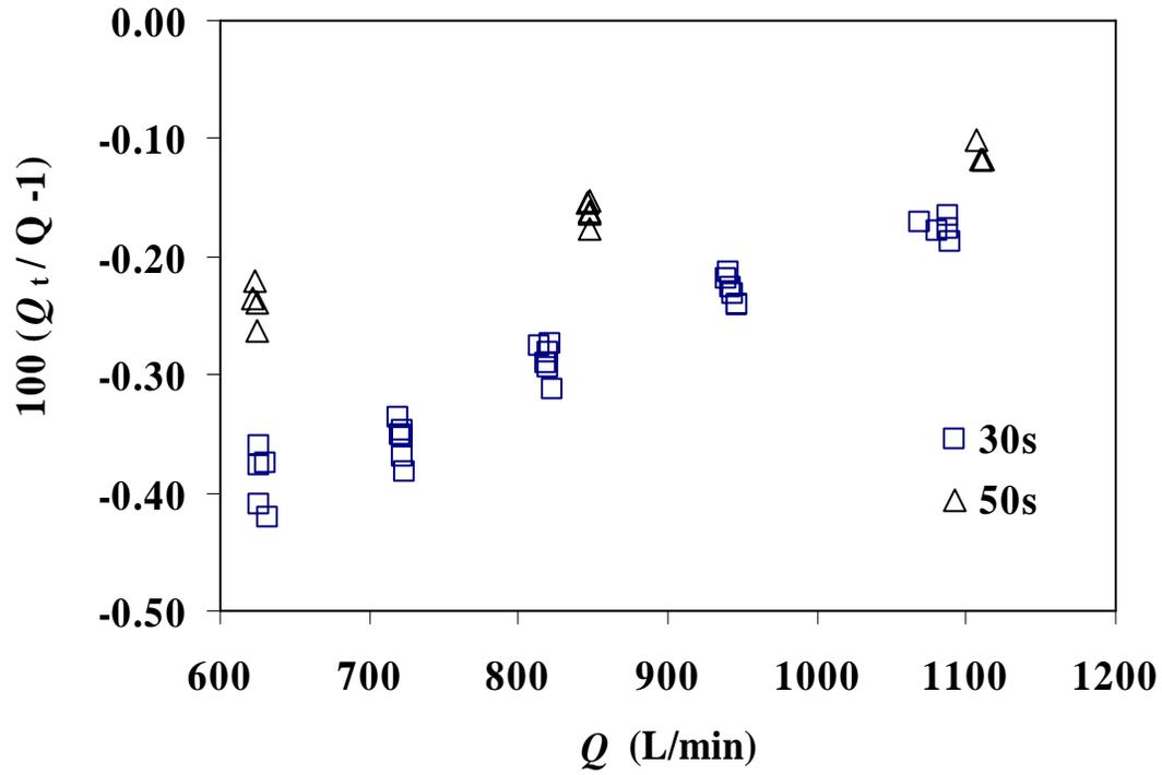
**Figure 11.** Differences between Traditional and Uni-directional Diverters, where No Correction is Made
