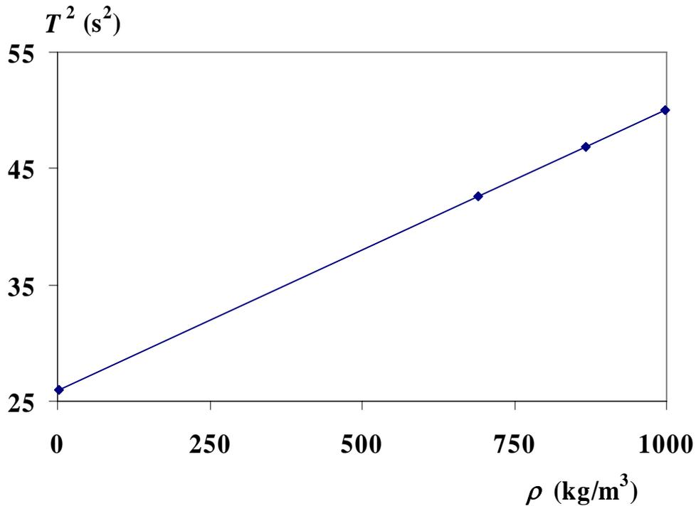
**Figure 15.** Densimeter Results Using the Four Fluids
