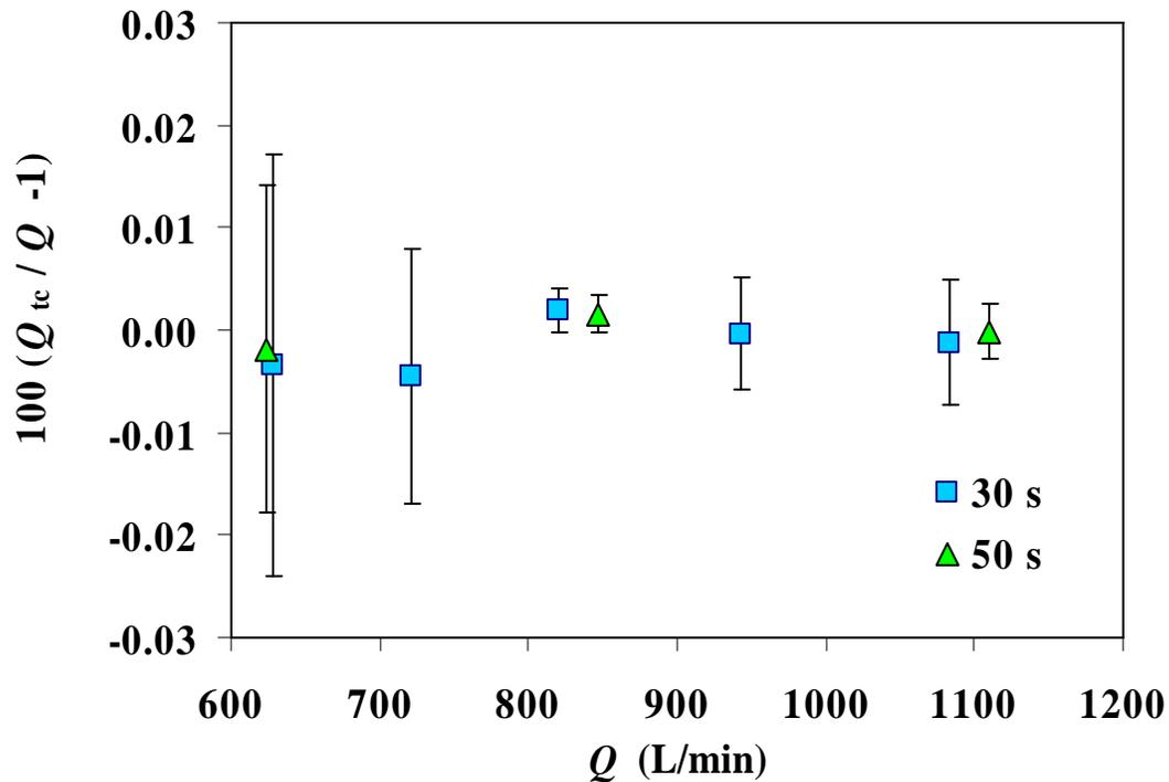
**Figure12.** Difference between Traditional and Uni-directional Diverter, where Time Correction is Included
