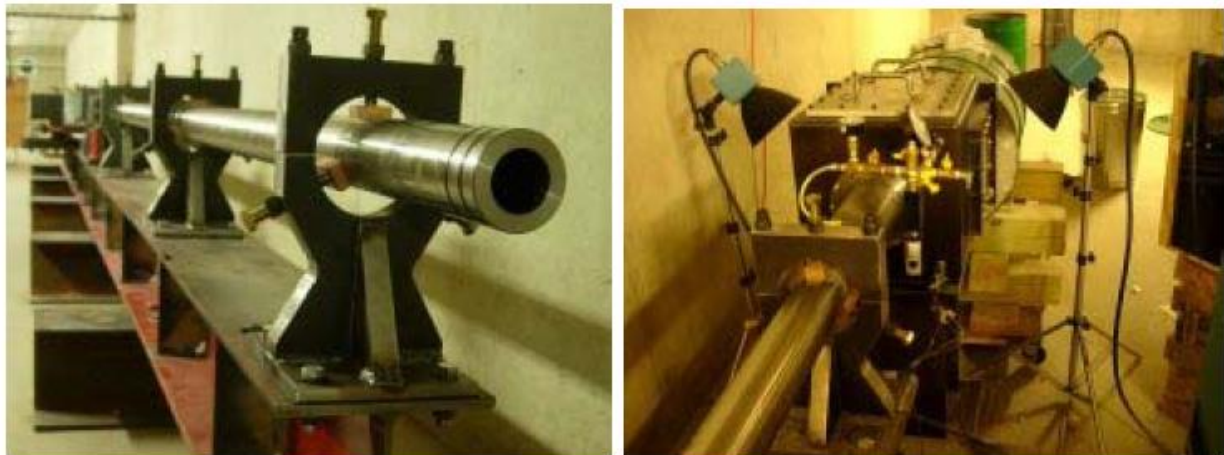
Figure 2: Gas gun system used in the study: Barrel (left) and target chamber (right).
