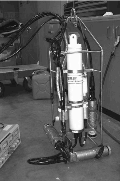
Figure 1: The three Dopbeams and a CTD unit mounted on the cage for deployment.
