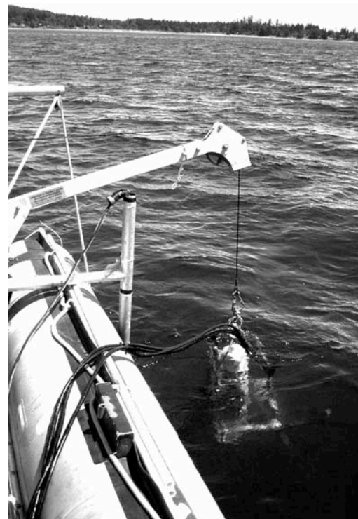
Figure 2: The instrument cage being lowered from a crane, which was mounted on the Zodiac.
