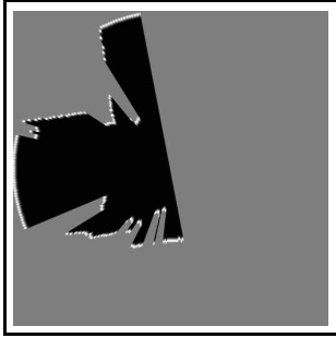
Figure 2: An example occupancy grid. The light areas are high-probability occupancy, and the dark areas are low-probability occupancy. The mid-grey areas are 50% occupancy, indicating no information about these cells.
