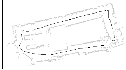
Figure 11: The map generated using corrected position estimates. The corrections were made using only the correction parameters \delta_{\text{trans}} and \delta_r , computed from the entire data set.
