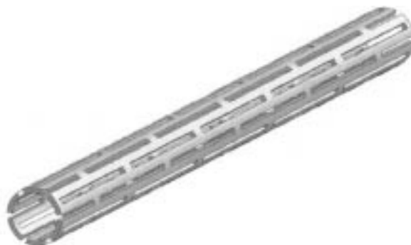
FIGURE 3 Original stent design: unexpanded configuration. The stent is assumed to be a tube of length, inner and outer diameters respectively equal to 16 mm, 1 mm and 1.2 mm. The tube has 5 rectangular slots in the longitudinal direction and 12 slots in the circumferential direction, each slot measuring 2.88 mm times 0.24 mm.
