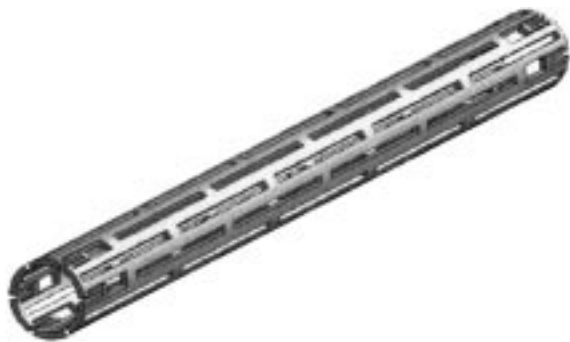
FIGURE 8 Modified stent design: unexpanded configuration. It is possible to note the added distal struts.
