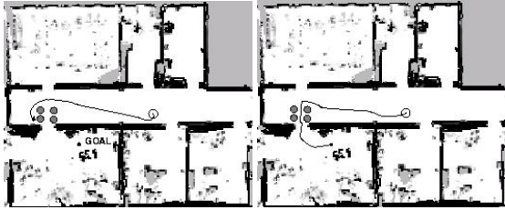
Figure 5: Albert tries to enter a doorway blocked by several obstacles using the DWA (left) and our technique (right).
