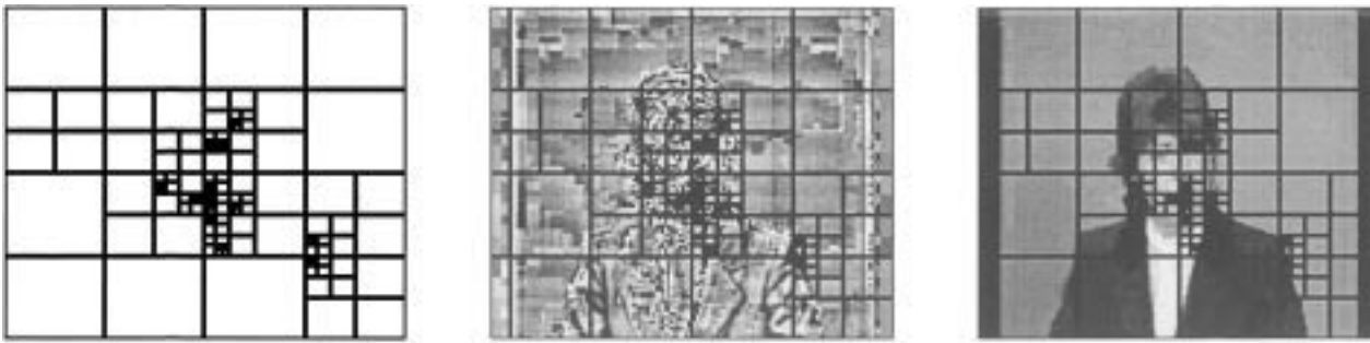
Fig. 9. QT segmentation example with and without overlaid MCER and original video frame [189].
