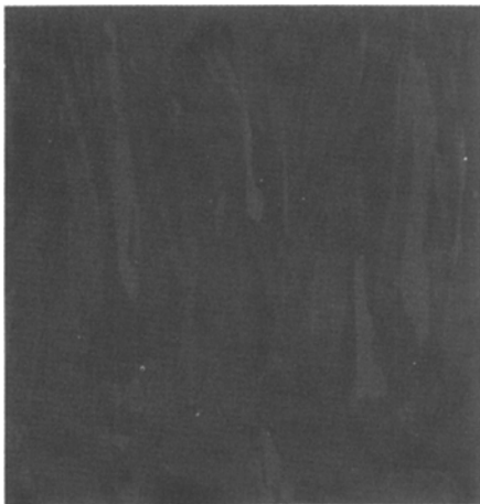
Fig. 1. Photograph of a polycrystalline wafer before polishing. Size: 2.5 \times 2.5 \text{ cm}^2 .
