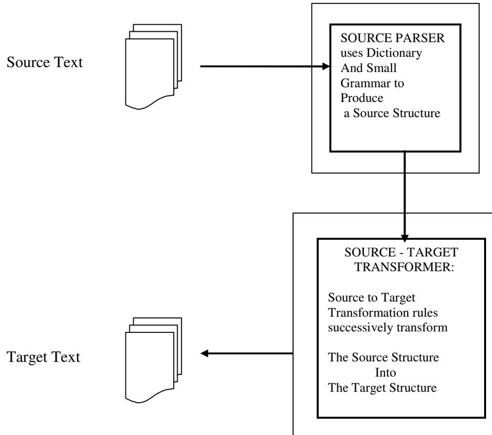
**Figure 2-3:** Transformer Architecture
