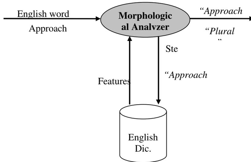
**Fig. 3-4** Architecture of the morphological analyzer
