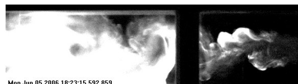
Figure 4-18 Combusting V-Gutter at 460F Inlet Temperature, Re = 9,700, Near LBO
