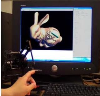
Figure 1: The haptic user interface.
