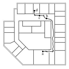
Figure 5: A measured trajectory that has been generated by the combination of four basic behaviors. a) Follow left wall. b) Follow right wall. c) Turn into right door. d) Stop.
