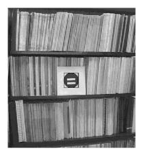
Figure 4: An artificial routemark. The square around the mark indicates that it has been recognized.
