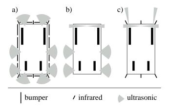
Figure 2: Illustration of the sensor subsystems of the wheelchair. a) Collision detection. b) Steering restriction. c) Navigation.
