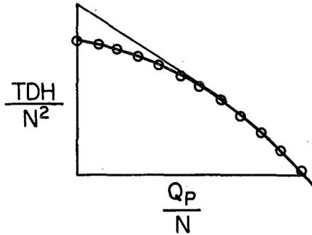
Fig. 13 Head-discharge curve for normal zone of pump operation
