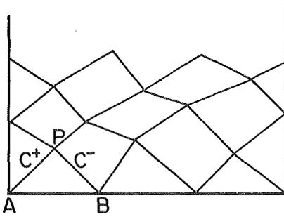
Fig. 8 Characteristics grid for high-velocity flow
