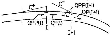
Fig. 14 Notation for calculation of cavity volume
