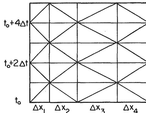
Fig. 4 Staggered grid for series pipeline, or for variable wave speeds
