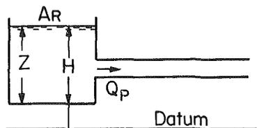
Fig. 7 Small reservoir at upstream end of pipeline
