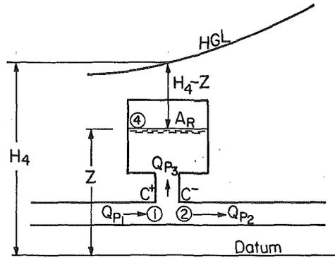
Fig. 15 Notation for an accumulator
