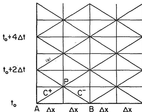
Fig. 3 Staggered rectangular grid
