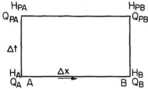
Fig. 5 Centered-implicit cell for a segment of pipe of length  $\Delta x$
