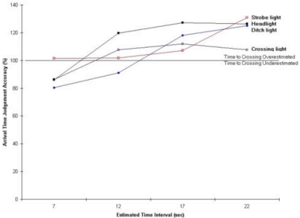
**Figure 7-1. Effect of Alerting Light System on Mean Arrival Time by Estimated Time Interval**
