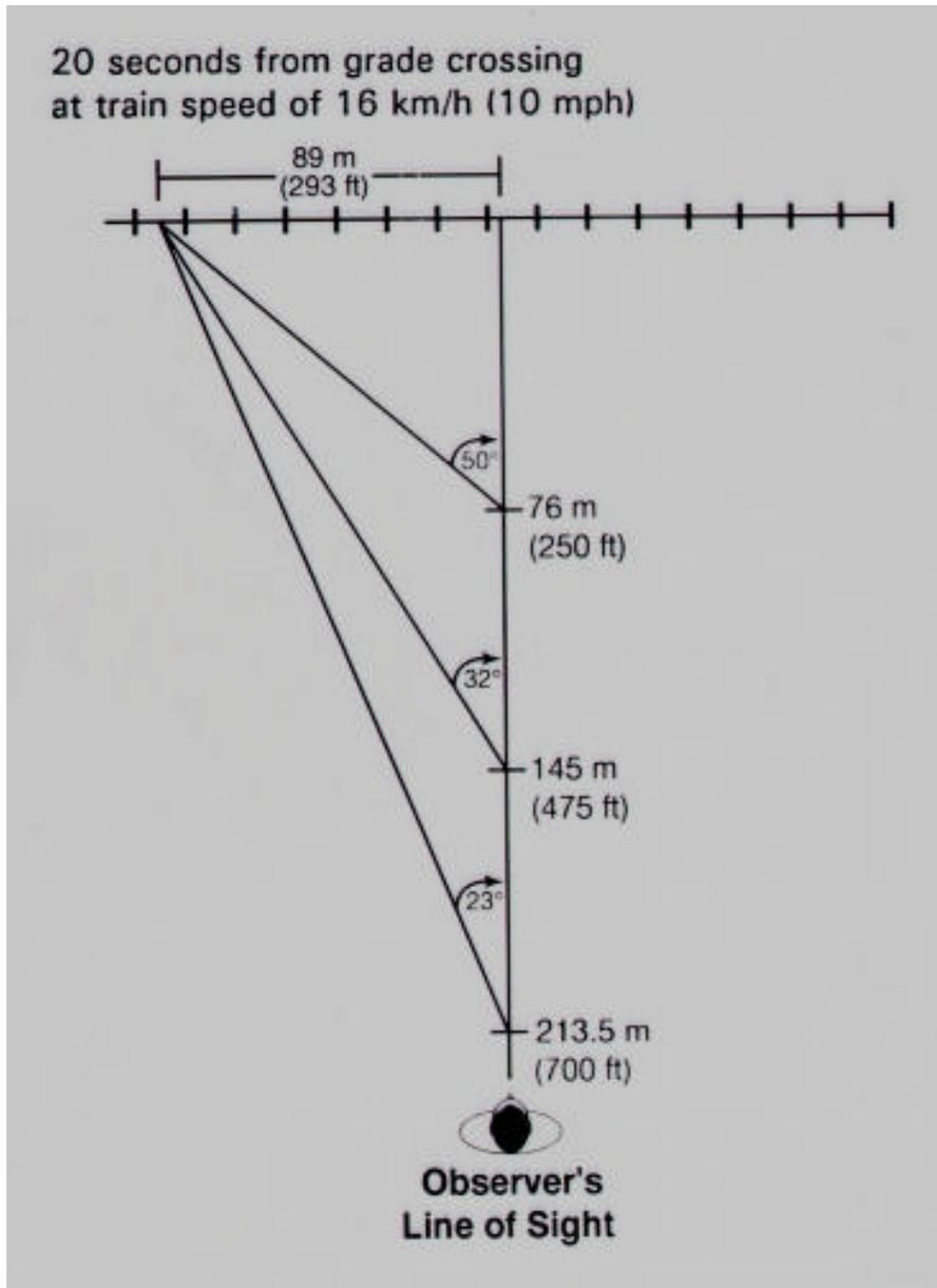
**Figure 2-2. Observation Angle as a Function of Distance from Grade Crossing**
