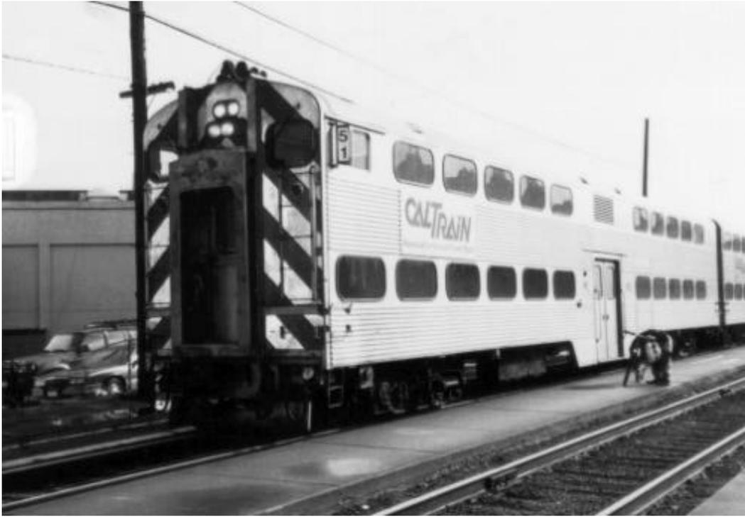
**Figure 6-2. CalTrain Train Cab-Car Not Equipped with Crossing Light System**
