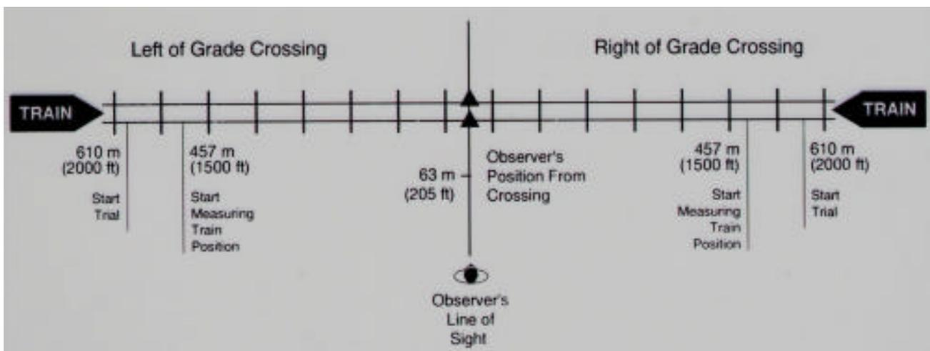
Figure 5-1. Field Test Site Layout and Observer Position
