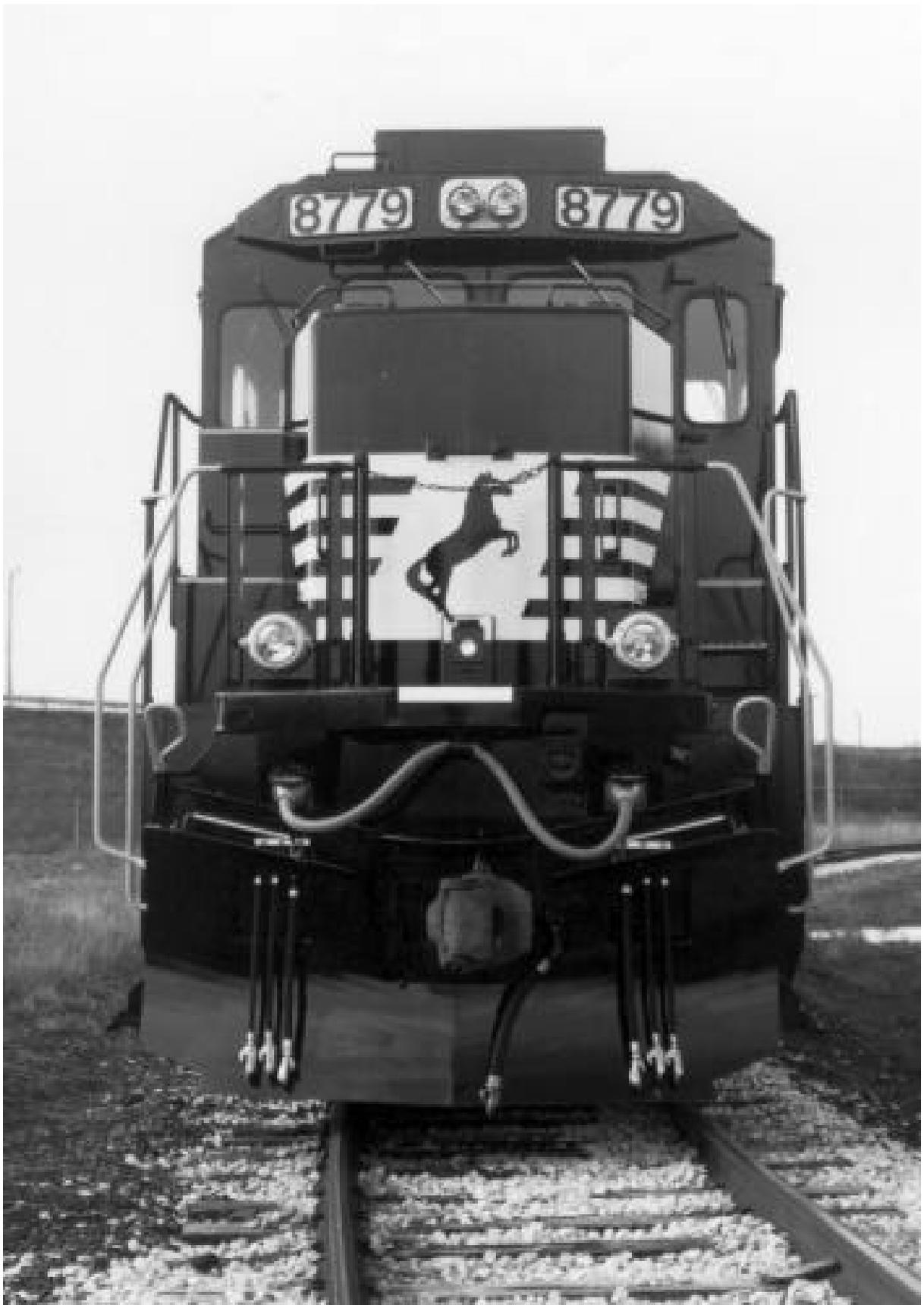
**Figure 6-4. Norfolk Southern Locomotive Equipped with Crossing Light System**
