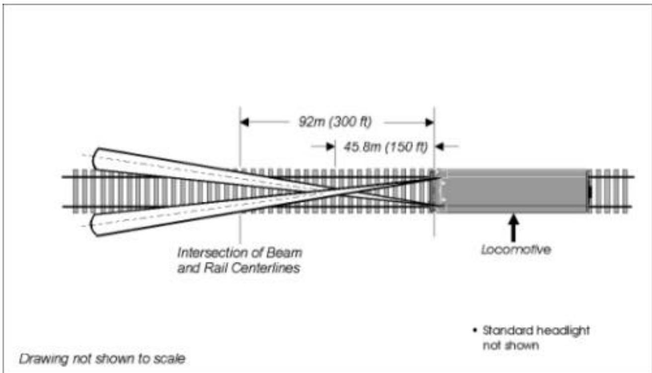
**Figure 3-4. "Canadian" Ditch Lights - Beam Focus Angle**
