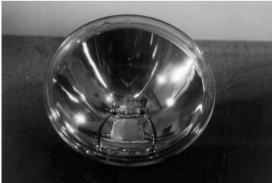
**Figure 4-1. 200-Watt PAR 56 30 V Locomotive Headlight**
