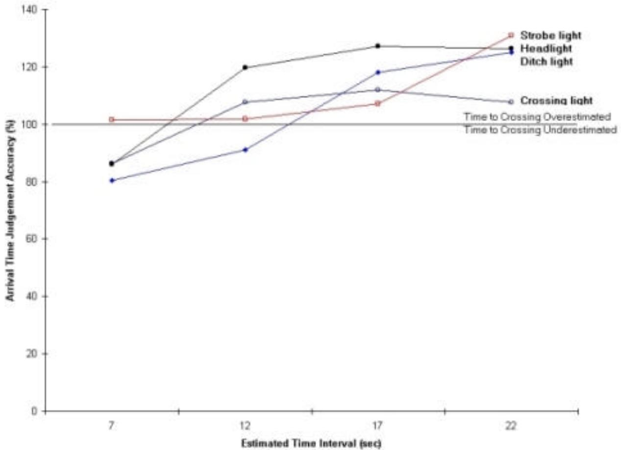
**Figure 5-4. Effect of Alerting Light System on Mean Arrival Time by Estimated Time Interval**
