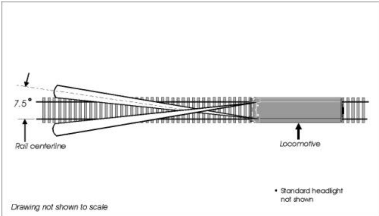
**Figure 3-8. Australian Alerting Light Beam Focus Angle**
