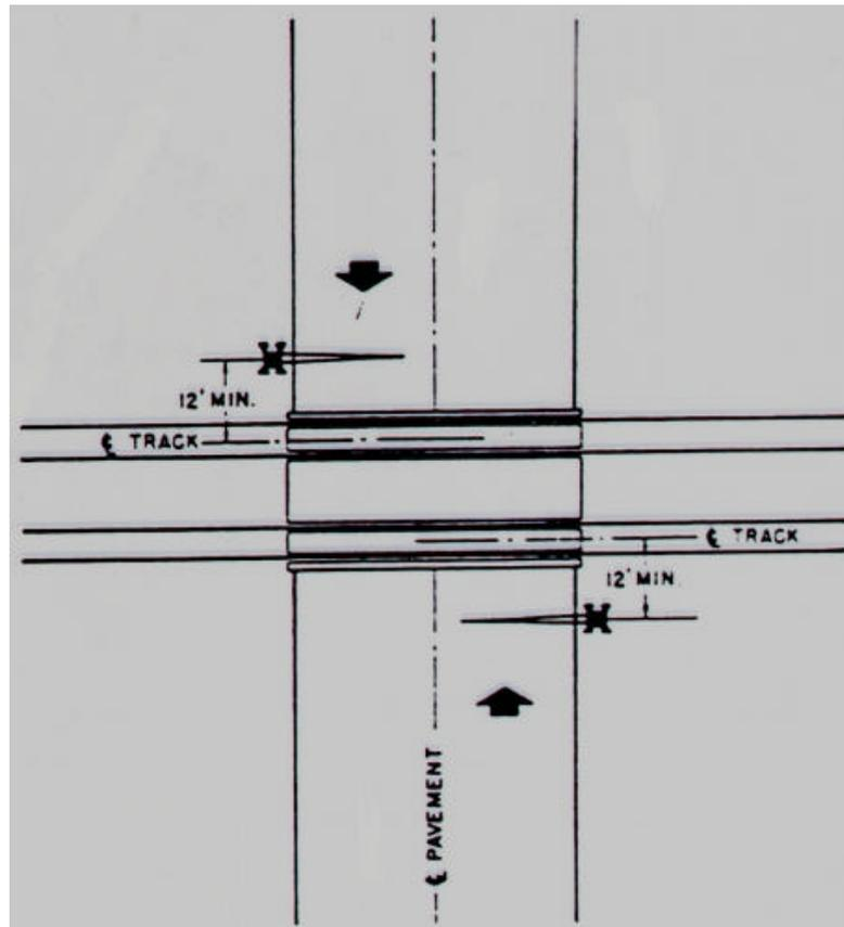
**Figure B-1. Grade Crossing at a Right Angle to Roadway**
