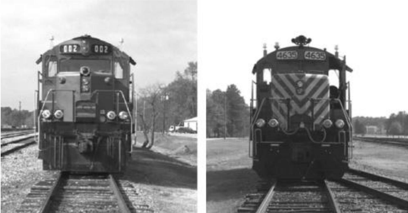
**Figure 5-2. Ft. Eustis Locomotives Equipped With External Experimental Alerting Light Systems**
