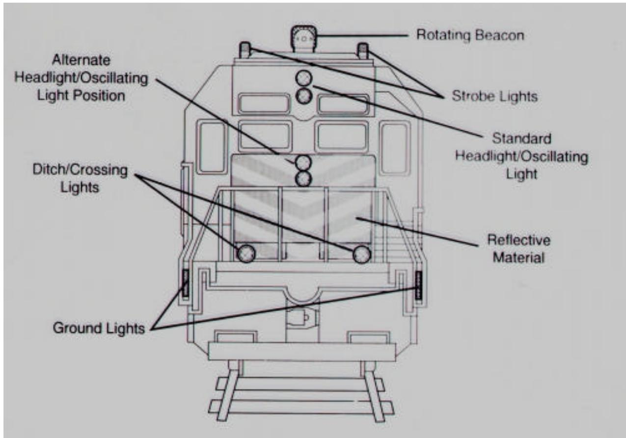
**Figure 3-1. External Locomotive Alerting Devices (Lights and Reflective Material)**
