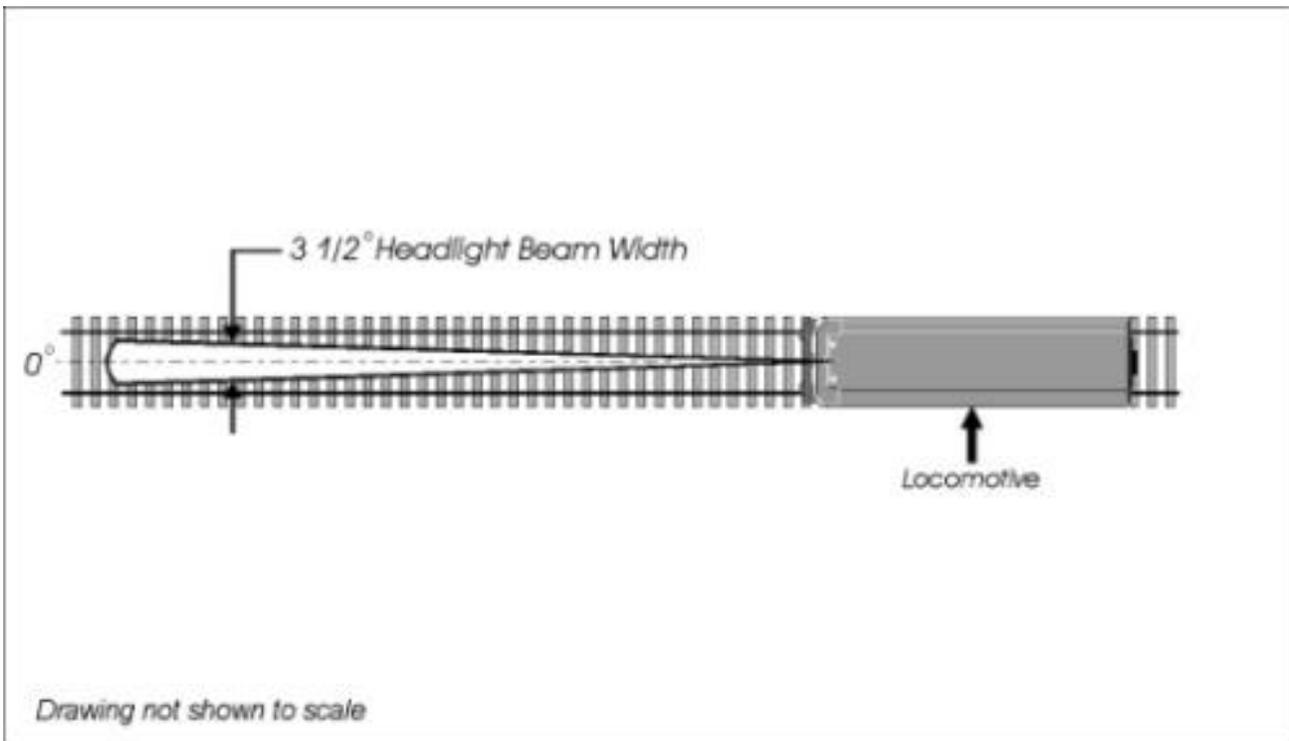
**Figure 3-2. Standard Headlight Beam Width/Focus Angle**
