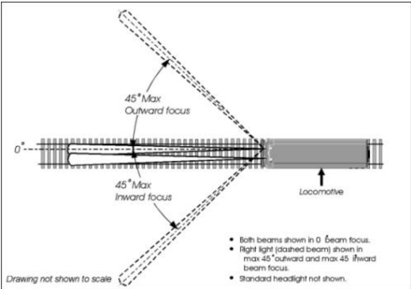
**Figure 3-5. U.S. Ditch Lights - Maximum/Minimum Beam Focus Angle**
