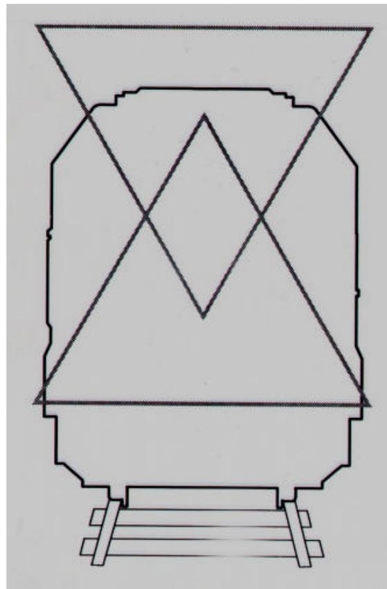
Figure 2-3. Triangular Locomotive Light Pattern
