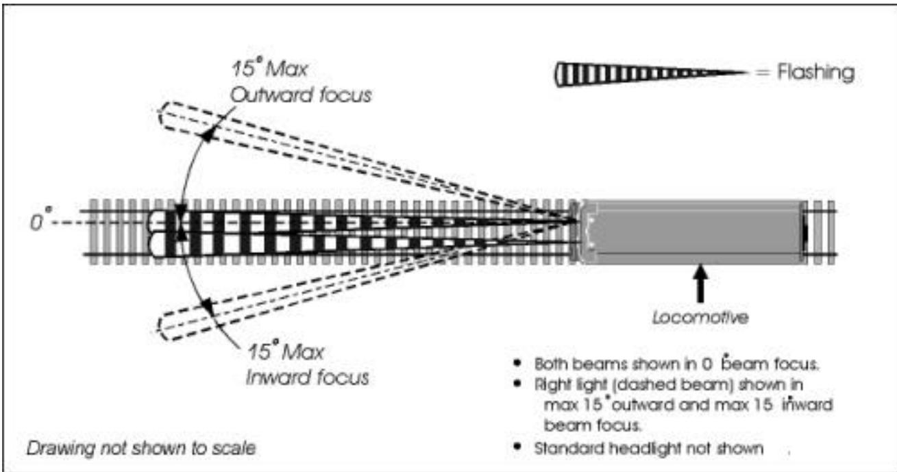
**Figure 3-6. Crossing Lights - Maximum/Minimum Beam Focus Angle**
