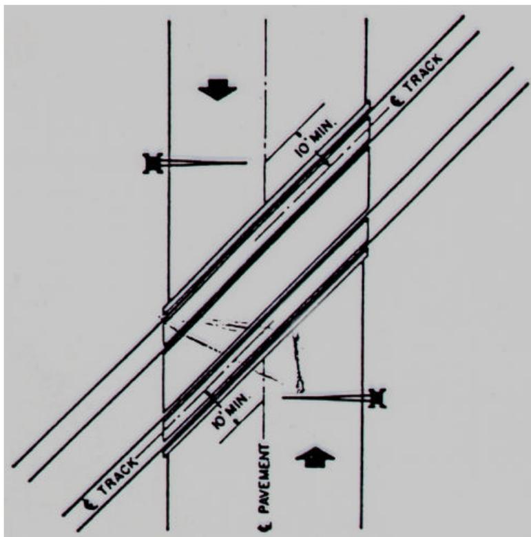
**Figure B-2. Grade Crossing at an Obtuse Angle to Roadway**
