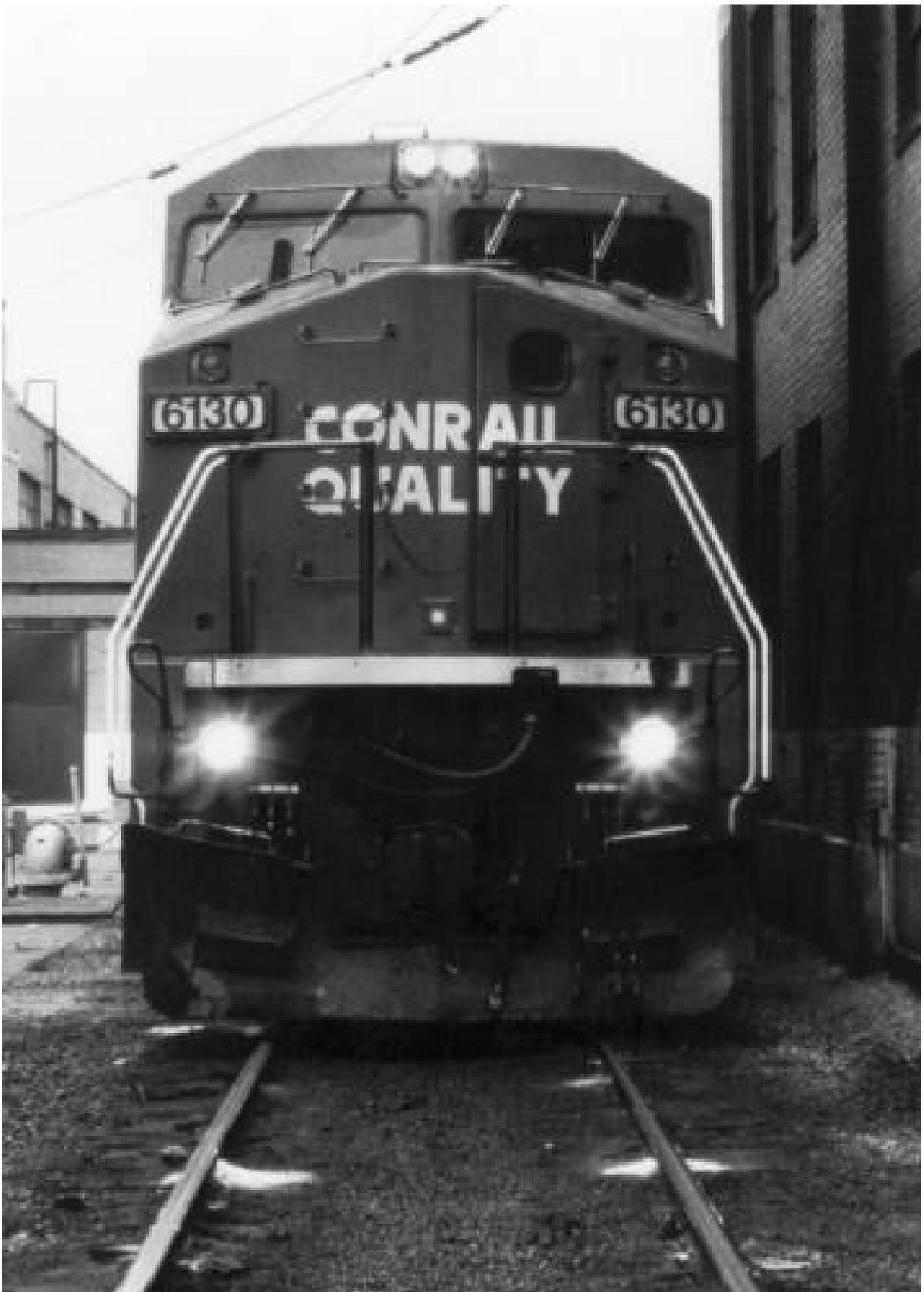
**Figure 6-3. Conrail Locomotive Equipped with Crossing Light System**
