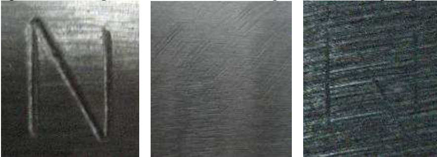
A. Original stamping number B. Number was obliterated C. Recovering results Fig. 5 Recovering “N” on vehicle frame sample 2 with etching reagent 3
