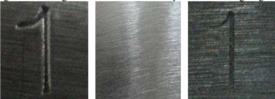
A. Original stamping number B. Number was obliterated C. Recovering results Fig. 6 Recovering “1” on vehicle frame sample 2 with etching reagent 3
