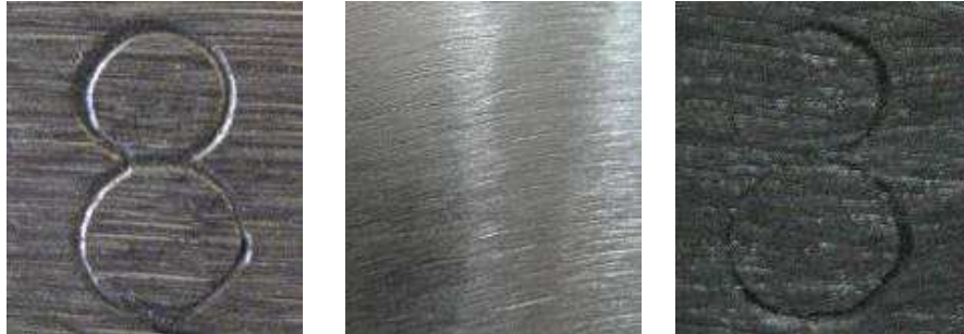
A. Original stamping number B. Number was obliterated C. Recovering results Fig. 4 Recovering “8” on vehicle frame sample 1 with etching reagent 1
