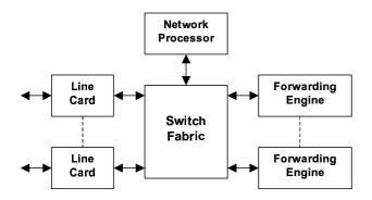
Figure 2: Architecture of a a high-speed router [10]
