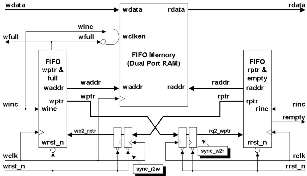
Figure 5 - FIFO1 partitioning with synchronized pointer comparison
