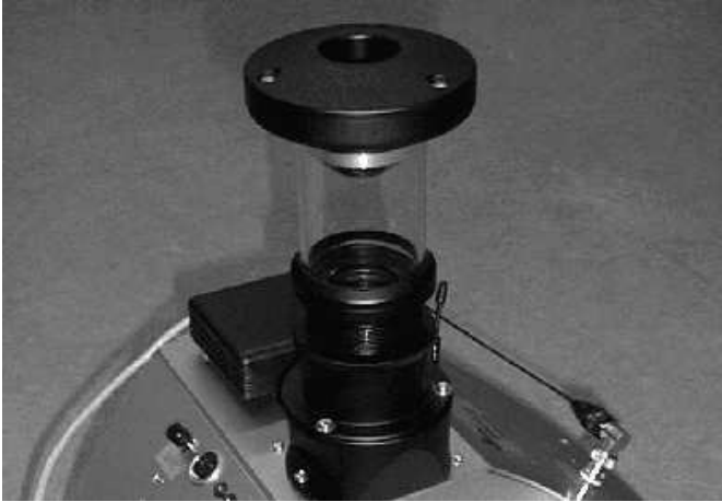
Figure 2: A robot with a panoramic camera mounted on the top. The actual camera is mounted at the bottom and “looks” upwards to the tip of a parabolic mirror, which in turn provides the panoramic scene. In this panoramic image, the horizon is somewhere between the circle’s center and its periphery. Some real-world, panoramic images can be found in [5].
