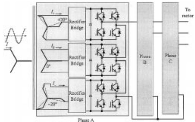
Fig. 26. Seven-level cascaded inverter with nonregenerative rectifier.
