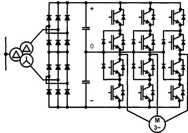
Fig. 24. Three-level diode-clamped inverter with 12-pulse input rectifier.
