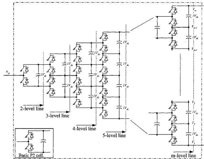
Fig. 6. Generalized P2 multilevel inverter structure.
