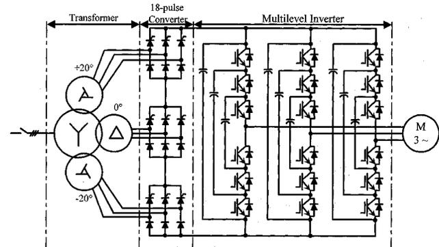
Fig. 25. Three-level capacitor-clamped inverter with 18-pulse input rectifier.
