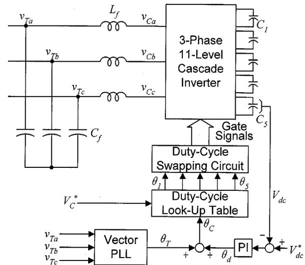
Fig. 21. Control diagram of the 11-level cascaded inverter.
