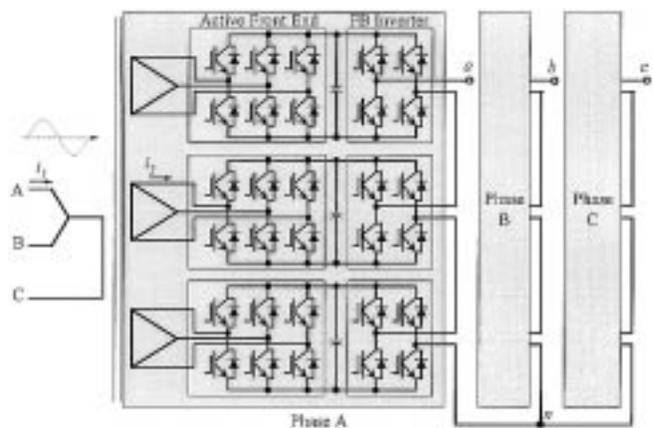
Fig. 30. Cascaded regenerative inverter with three-phase AFEs.
