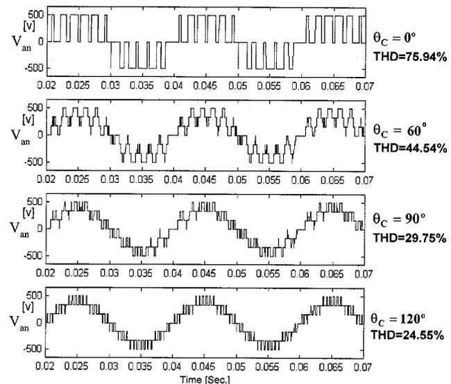
Fig. 14. Total voltage of three cells in series connection for different phase displacement in the carriers.
