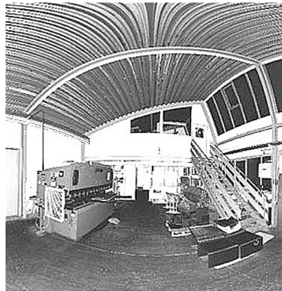
Figure 3: The figure shows a reflectance image. There is a one to one correspondance between the reflectance image and its complimentary image, the range image.
