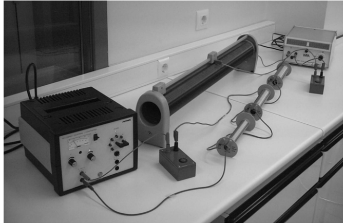
Figure 3. Experimental set-up to verify the conditions for Faraday's law.
