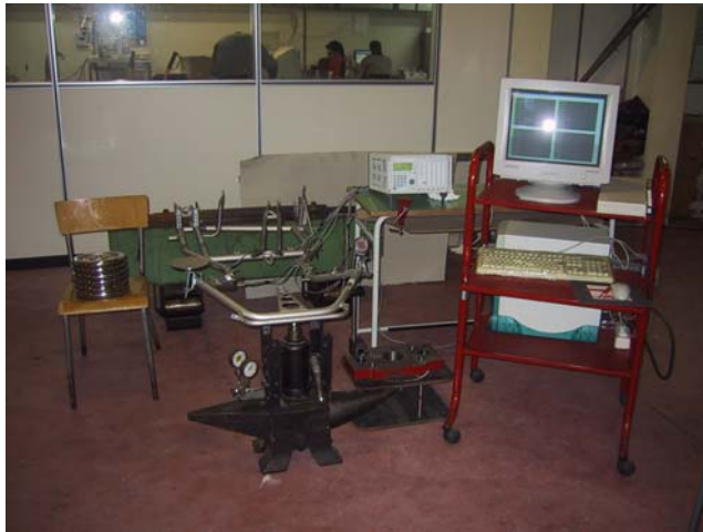
FIG. 8: The experimental set up adopted to analyze the frame level of deformation under static loads.
