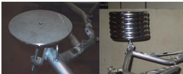
FIG. 9: To apply the loads, a circular plate mounted on the left front tire support of the frame was used.
