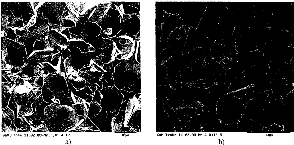
Figure 3. SEM pictures of two GaN samples, both deposited at 1000 °C on silicon. a) with propylamine addition, b) without propylamine addition.
