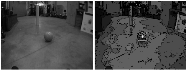
Figure 4: The left image shows a raw image in an indoor scene, the right the resulting regions, with the identified ball region and yellow marker outlined with a bounding box.
