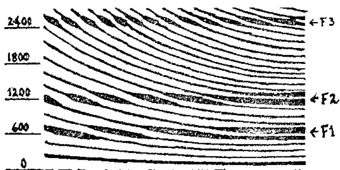
Fig. 3--A spectrogram of a showing that voice pitch can be independent of vowel color: The voice melody frequency falls by about one octave (about 240 cps to 120 cps), but the formant frequencies of a (about 700, 1200, and 2400 cps) remain unchanged throughout.
