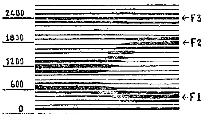
Fig. 4--A spectrogram of a-eh showing that vowel color can be independent of voice pitch: The frequencies of formants one and two change from about 700 cps and 1200 cps for a to 500 cps and 1800 cps for eh but the voice melody frequently remains unchanged at about 110 cps throughout.
