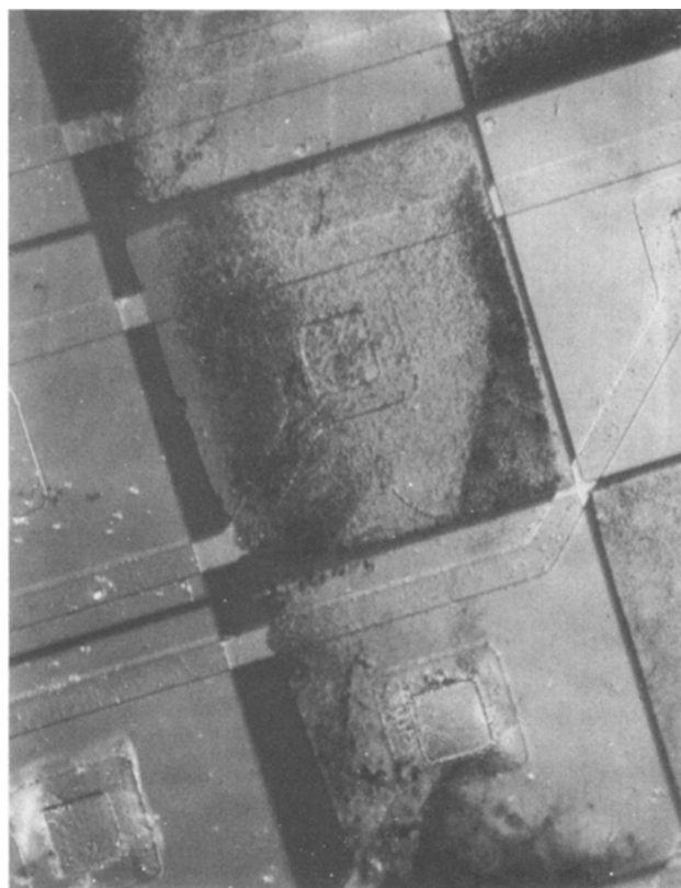
Fig. A-2. Segments of an "old" micromosaic electrode
