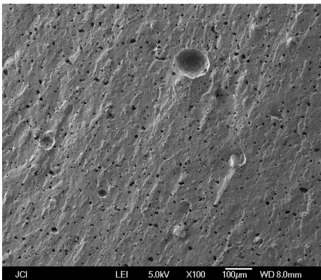
Fig.3 The scanning micrograph of the sintered body
