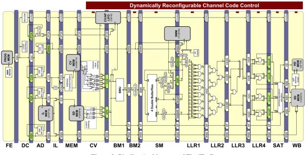
Figure 2: Pipeline Architecture of FlexiTreP
