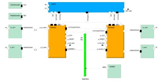
Figure 3: Example Platform with 2 ASIP Cores
