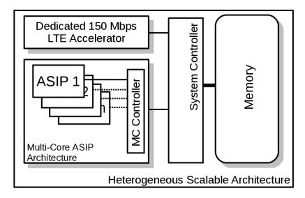
Figure 1: Example of a Heterogeneous Scalable Channel Decoding Architecture [14]
