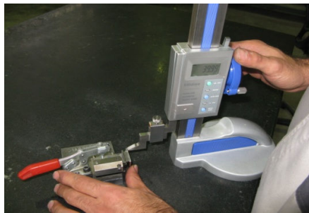
Fig 1.3. measurement of the rotation parameter using a height gauge by the operator
