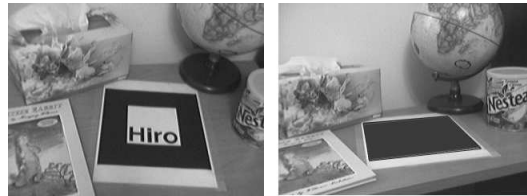
Figure 7. ARToolkit marker in the scene (left). Virtual square, superimposed onto the marker during tracking (right).
