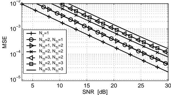
Fig. 7. MSE vs SNR for various antenna sizes  $N_T = N_{Tf}N_{Tt}$ , for channel B and parameter set (b.) from Table II.
