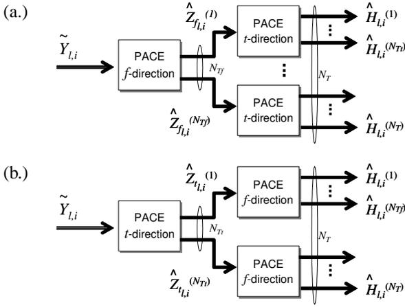
Fig. 3. Principle of  $2 \times 1\text{D}$  PACE type I (a.) and type II (b.), for OFDM systems with multiple transmit antennas.
