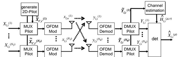
Fig. 1. Block diagram of the OFDM system with  $N_T$  transmit antennas.
