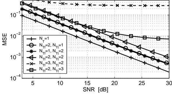
Fig. 6. MSE vs SNR for various antenna sizes  $N_T = N_{Tf}N_{Tt}$ , for channel A and parameter set (b.) from Table II.
