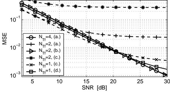
Fig. 5. MSE vs SNR for channel A, with different pilot spacings,  $D_f$ ,  $D_t$ , and various subset sizes  $N_{Tf}$ ,  $N_{Tt}$ .  $N_T = 4$ .
