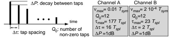
Fig. 4. The power delay profile of the used channel model.
