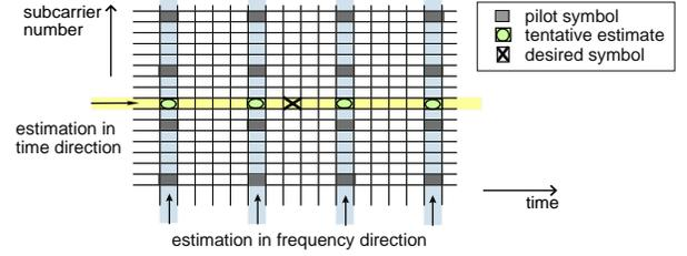
Fig. 2. Principle of  $2 \times 1D$  pilot aided channel estimation (PACE).
