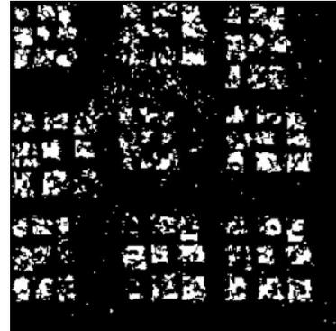
Figure 4: Pattern image recovered after StirMark randomization and bending
