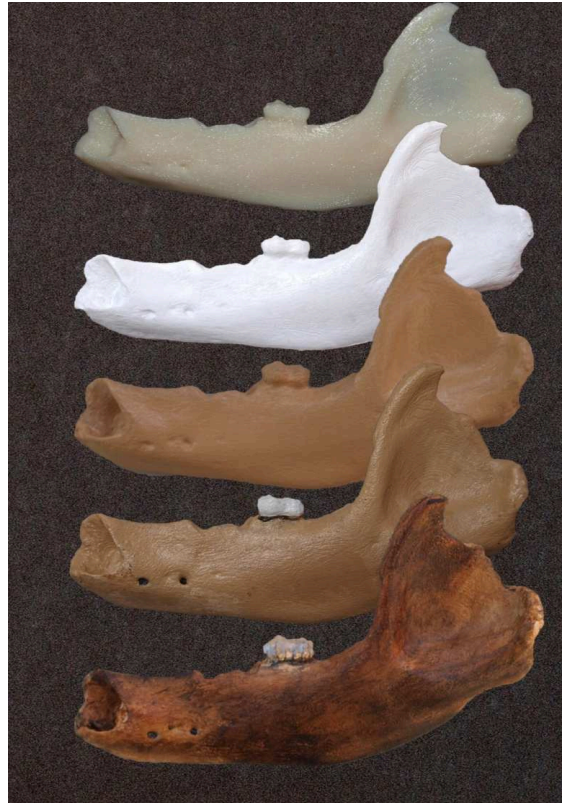
Fig. 9. Physical model of the entire part made of ABS (top) and thereafter acrylic coatings and paints applied on the part to match the exact colour of the paleontological find.
