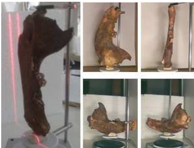
Fig. 2. Laser scanning of jaw-bone and different positioning during scanning
