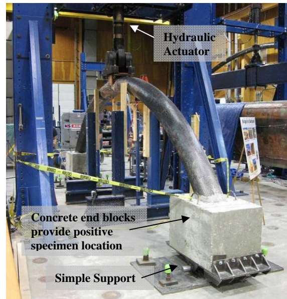
Figure 4. Arch Test Setup
