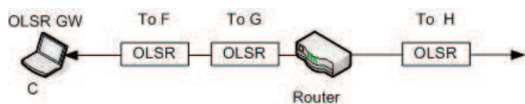
Figure 5.5: Sending and receiving OLSR messages via unicast communications at node C of Fig. 5.4
