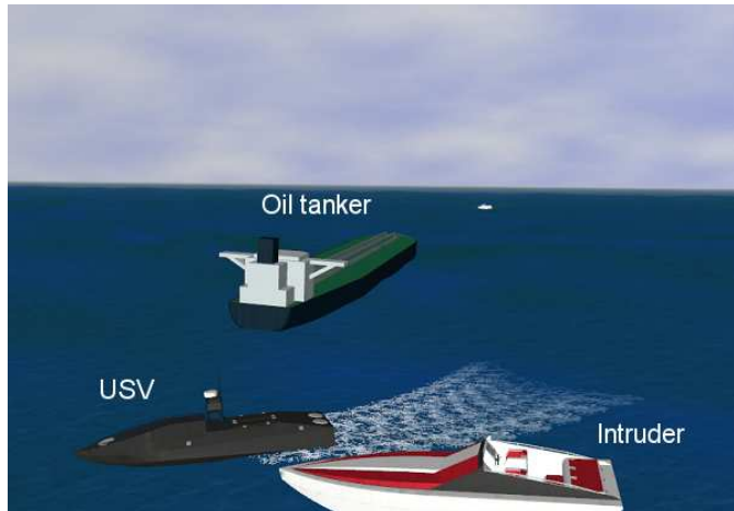
Fig. 1: Virtual environment: Unmanned Surface Vehicle (USV) is protecting an oil tanker by blocking the advancement of an intruder boat
