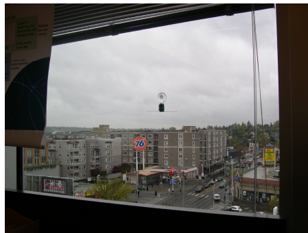
Fig. 6. WISP mounted by suction cup to interior window for light level measurement experiment
