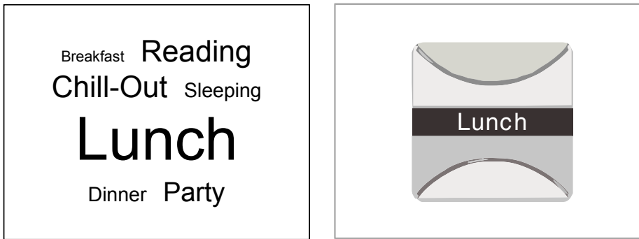
Fig. 3. Scene cloud and display-enriched switch as different user interfaces for scene control in a smart home environment. The most probable next scene, Lunch , is highlighted.
