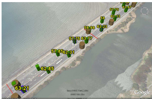
Figure 9: Satellite image of the first experiment site I-80 near Berkeley, CA. The red lines represent the locations of the VTLs, the blue squares show the speed recorded by the VTL, the green squares represent the position and speed stored in the phone log. The brown circles represent the readings from the vehicle speedometer.
