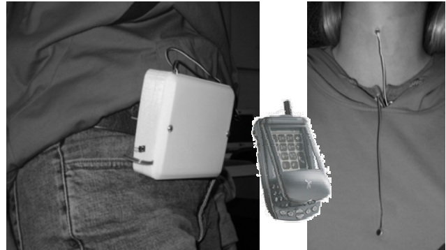
Figure 1. SenSay: sensor box mounted on the hip (left), the mobile phone (center), and voice and ambient microphones mounted on the user (right).
