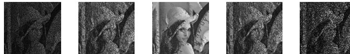
Figure 6. a) Noisy image with 0% Salt, 70% Pepper Noise & PSNR of 7.20. Restriction results obtained for b) 'X1' with PSNR of 10.95 c) 'X2' with PSNR of 13.24 d) 'X3' with PSNR of 11.25 e) 'X4' with PSNR of 10.02.
