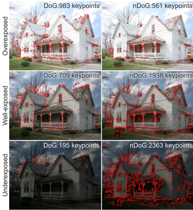
Figure 4. The location and number of extracted keypoints for nDoG and DoG, in a scene captured with different exposures.
