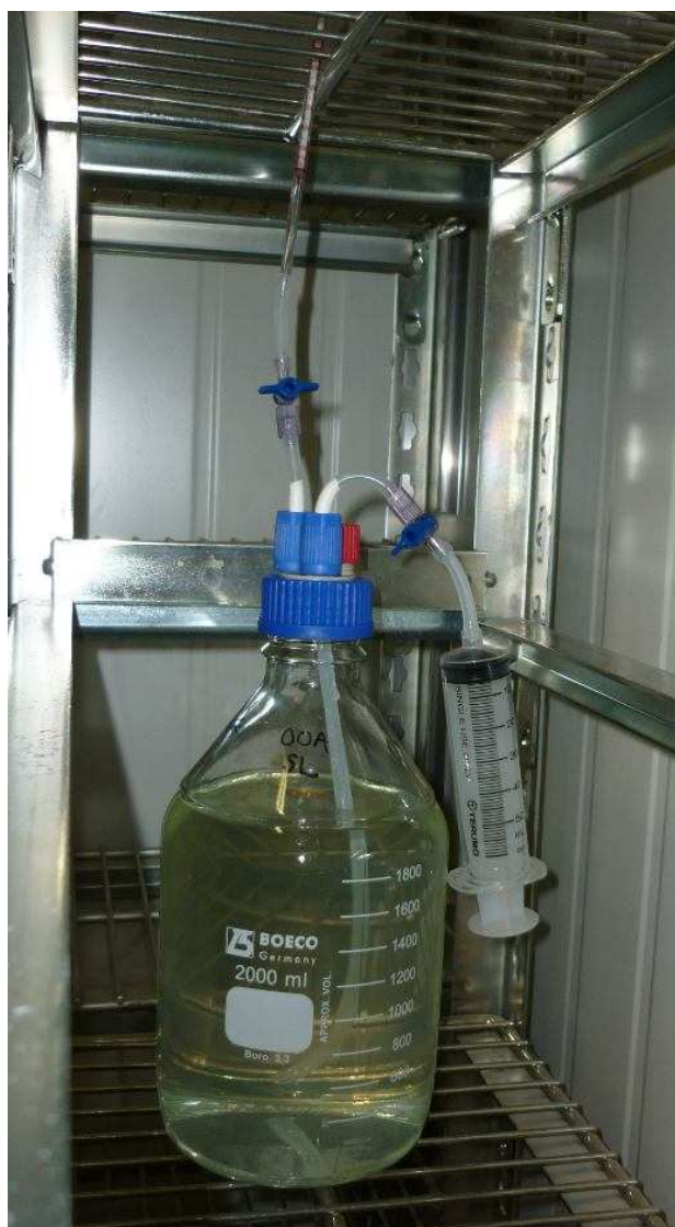
Figure 2.1. Photograph of the lab-scale wine fermentation setup before inoculation, showing the H 2 S detection tube outlet on the left and the sampling tubing on the right.
