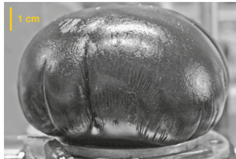
Fig. 15. The chamber size is 20 L and the membrane is not prestretched. Voltage is ramped up and is then kept at 5.5 kV for several minutes. The membrane forms wrinkles and clefts.
