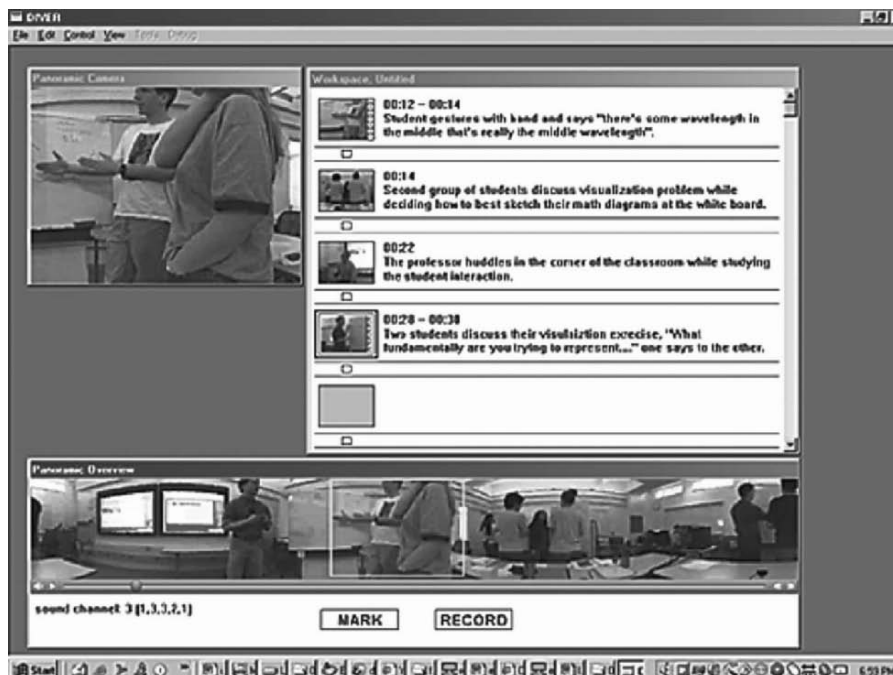
Figure 3. DIVER's windows: (1) overview ("Look") at bottom, (2) magnified viewing ("Notice") at upper left, and (3) the Dive worksheet ("Comment") comprised of panels.
