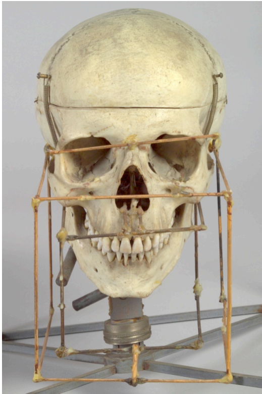
Figure 1.2 Porionkubus. A system to perform three dimensional measurements on a face or skull with fixed reference points. From the dentistry collection, University Museum Utrecht, The Netherlands.
